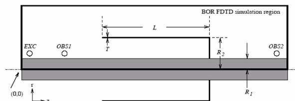
**Figure 1** BOR FDTD Structure for the calculation of balun isolation characteristics.
