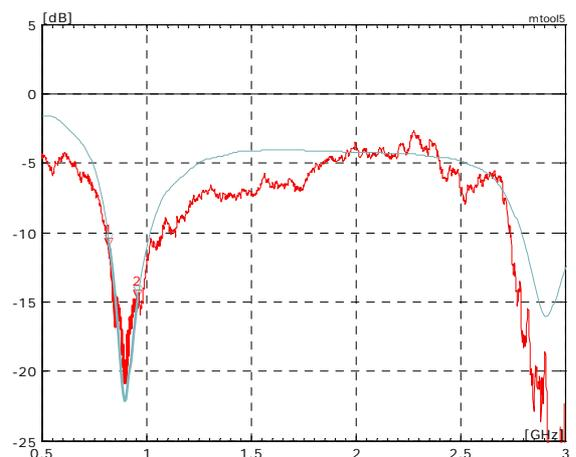
**Figure 2** Measured (thick line) and Simulated isolation characteristics for an 890 MHz balun
