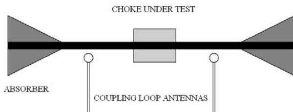
**Figure 3** Experimental configuration for isolation measurement of chokes on cables.
