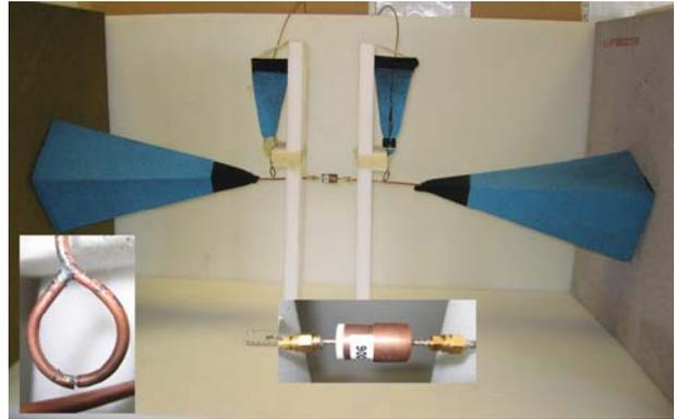
**Figure 4** Photograph of balun measurement fixture with probe and balun inset shown.
